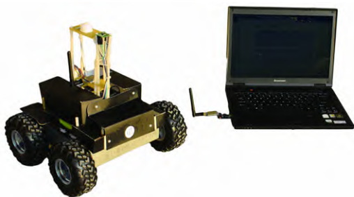
图 2 道路照明效果检测机器人实物图 Fig.2 Real image of the road lighting effect detection robot
